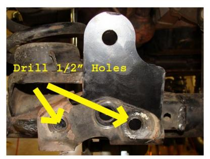
• (3.5" MAX TRAVEL / 5.5" X-FACTOR) Install the supplied front track bar support bracket to the factory bracket and our track bar bracket as shown below using the supplied ½" x 3" bolts, ½" washers, and ½" nyloc nuts.
