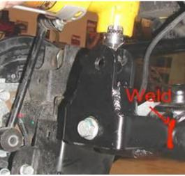
• (ALL X-FACTOR KITS / 3.5" MAX TRAVEL) Install the rear upper control arms set to the specified length for your kit according to our measurements and secure using the OEM hardware.
