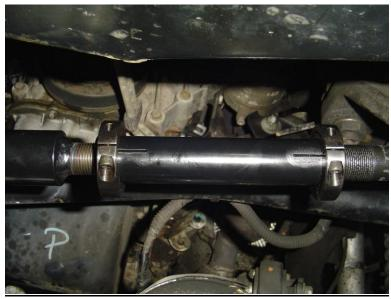
Quick adjuster with shaft collars installed
