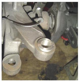
• Insert the split steel tapered sleeve into the knuckle as shown above.
