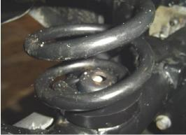
**Note:** A simple and cost effective way to retain the rear coils to the axle is to use a hose clamp up through the center hole of the spring pad and clamp it around the bottom winding of the coil spring.
