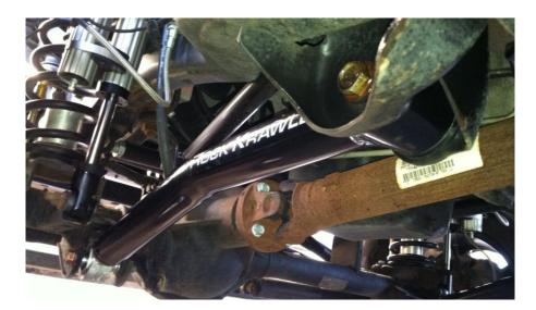
• (3.5" MAX TRAVEL / 5.5" X-FACTOR) Install the supplied front track bar bracket into the factory track bar bracket on your axle. Secure it using the OEM lower track bar hardware. Then drill out the other two holes in the OEM bracket through the supplied bracket with a ½" drill bit.
